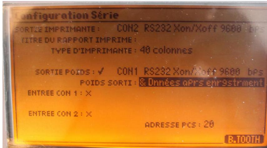
Connect your cable on COM 1 on the scale head. You must use a NULL MODEM cable and an USB adapter to connect to the PC. (or an adapter USB null modem). *The cable of adaptation USB is normally not provided with the scale.* If you buy one of them, it is suggested getting to you a model with the FTDI "Chip set" and ensure you that it is compatible with your version of Windows.
