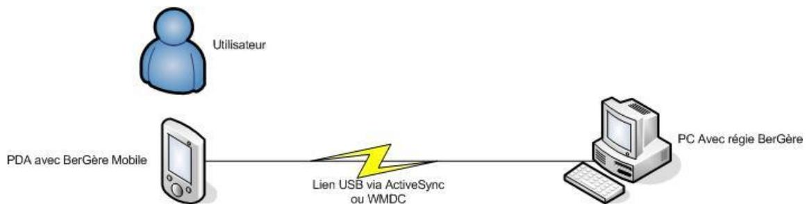
The Synchrobergère software is the PC based application that transfers files containing data from one device to the other, in both directions.
